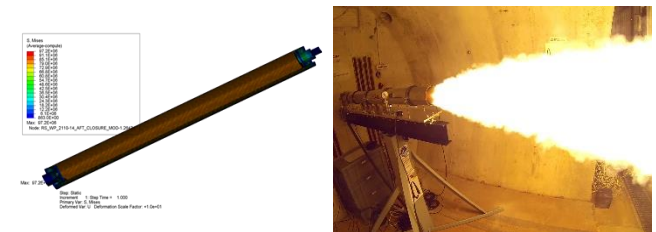
Solid Rocket Motor FEM Analysis and Rocket Motor Test
